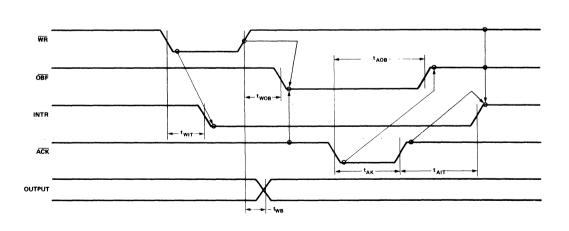
Figure 9. Mode 1 (Strobed Output)
